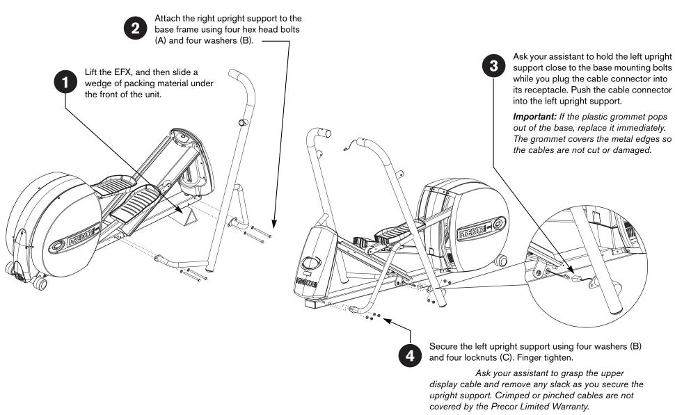
Hold the display console above the upright supports, and then plug the cable connector into its receptacle. Push excess cable into the upright support.
